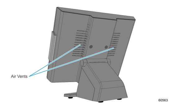
Do not place the terminal in an enclosed area where sufficient ventilation is not available. Leave at least 100 mm (4 inches) of clearance from air vents.
