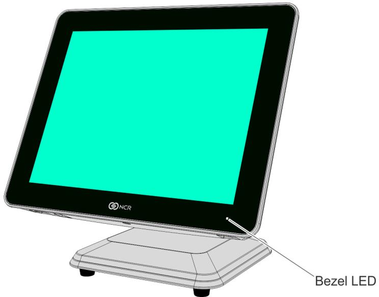
The Front Panel Bezel LED has multiple functions as defined below.
