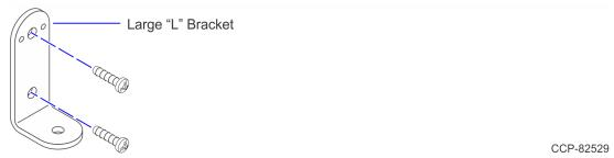
b. Install the Mount Cup on the Large "L" Bracket using the 3/8-16 x 7/8" Button Socket Cap Screw and 3/8-16 Nylon Stop Nut.
