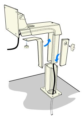
Slide the Side Cover onto the lower half of the Checkstand Base.
