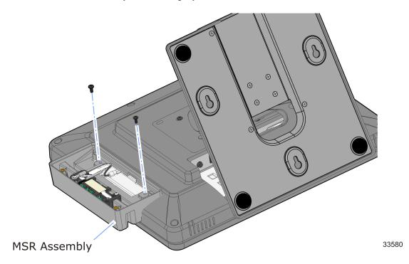
5. Install the MSR Rear Cabinet on the MSR Assembly (2 screws).
