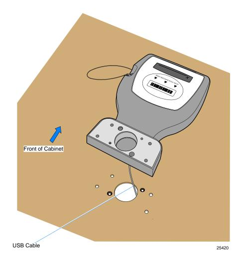
7. Insert the supplied 10-32 x 2 in. hex bolts (2) through the inner holes in the Mounting Plate, Signature Capture Base, and countertop.
