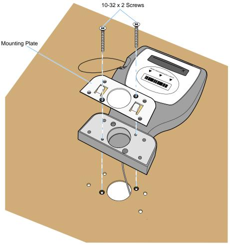
8. Place the Bolt Plate (removed earlier in Step #2) under the countertop and thread the screws through it. Secure the Mounting Plate to the predrilled holes in the countertop, using the appropriate type screws for the two *inner* holes.
