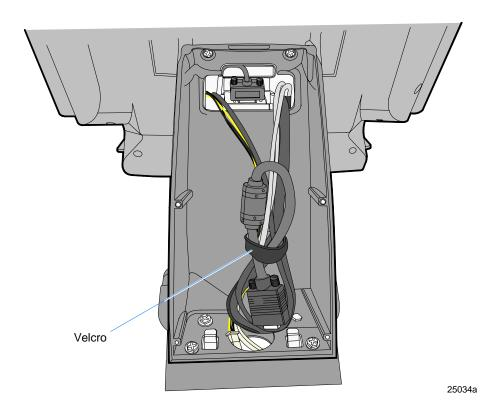
13. Install the Column Cover. Slide the upper tab into the slot and secure it with screws (2) in the bottom.
