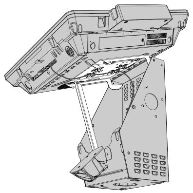
8. Install the Cable Cover on the terminal (use the same three screw holes that were used to mount the previous scanner assembly.
