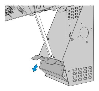
6. Hook the bottom of the Scanner Faceplate onto the bottom edge of the opening on the Fixed Angle Mount and then secure the assembly with screws (2).
