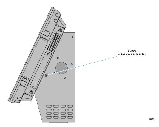
b. Tilt the display as shown and rest the display on the Display Support.
