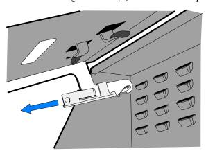
f. Remove the display from the Fixed Angle Mount.
