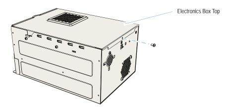
7. Slide the top slightly toward the end of the unit as shown and then lift it up to remove it from the Electronics Chassis.
