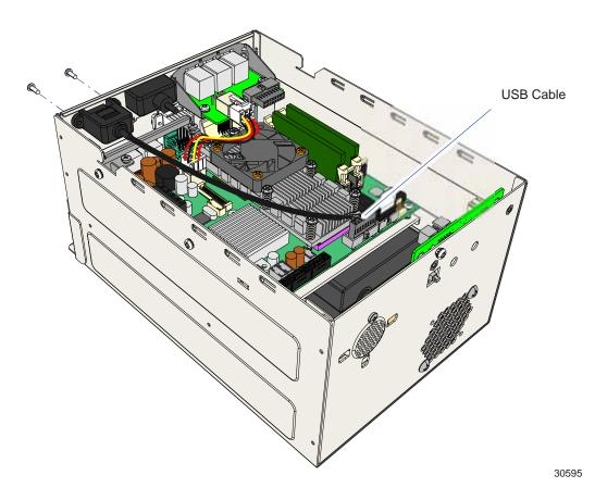
13. Install the new USB Cable to the Extended I/O Card, Motherboard (Header), and Back Panel (2 screws).
