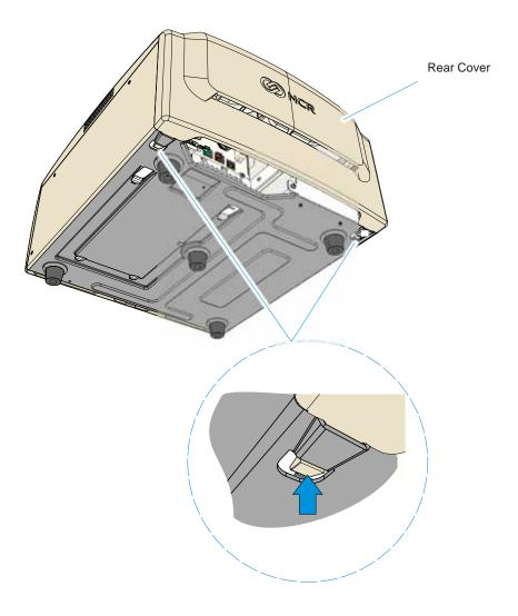
b. Pivot the bottom of the cover out as shown to remove it.
