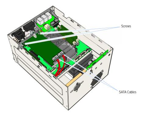
c. Disconnect the RAID Card from the Riser Board.
