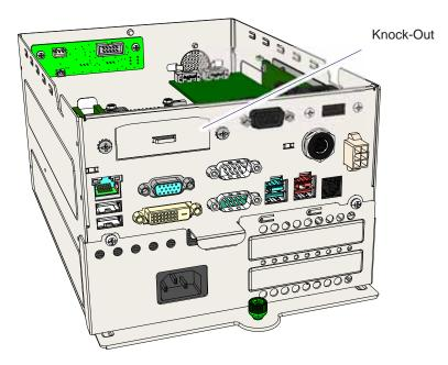
9. Temporarily remove the RAID Card so the Extended I/O Daughter Card Power Harness can be connected to the Motherboard.
