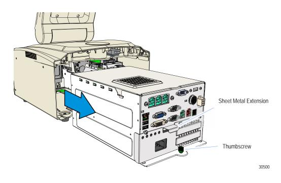
6. Remove the screw that secures the Electronics Box Top.
