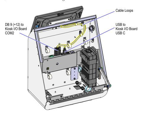
7. Route the Display Port Cable through cable loops and then connect to the NCR 7709 Port. Ensure that cables are secured with cable ties as shown in the image below.
