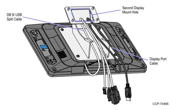
5. Install the Second Display Assembly to the NCR 7709 kiosk. For more information, refer to *Installing the Second Display Assembly* on the facing page.
