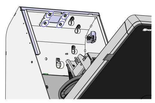
4. Insert the Second Display cables through the NCR 7709 hole as shown in the image below.
