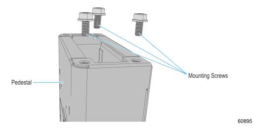
8. Position the kiosk on top of the pedestal with the Mounting Screws (3) extending up through the keyholes in the bottom of the kiosk cabinet. Slide the kiosk to the right.
