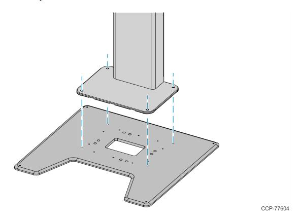
3. Secure the pedestal with four M8x20mm screws and four washers.
