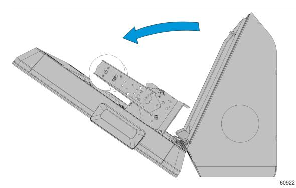
2. Install the PIN pad blank plate.
