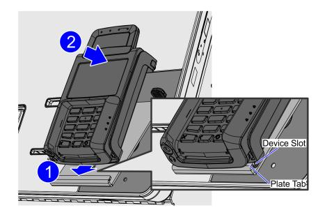
b. Tighten the M3 screw to secure the PIN Pad to its Mounting Bracket.
