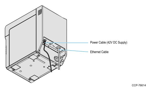
7. Connect the Ethernet cable to the LAN.
