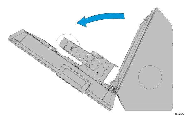
2. Install the coupon blank plate. Secure with screws (2).
