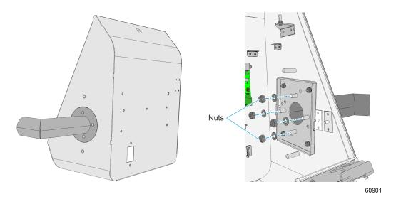
4. Re-install the power supply bracket and power supply.
