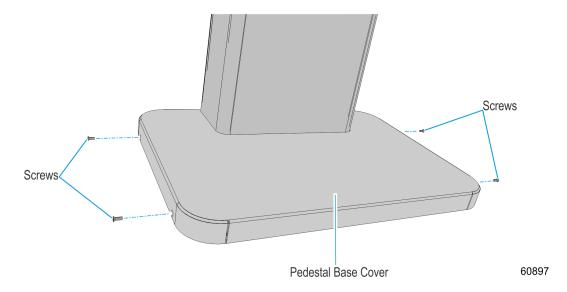
7. Install the Mounting Screws (3) on the pedestal. Partially tighten the screws,, leaving room for the kiosk cabinet to slide under the screw heads and lock-washers. Use a **6** mm (15/64 in.) Allen Key to drive the screws.
