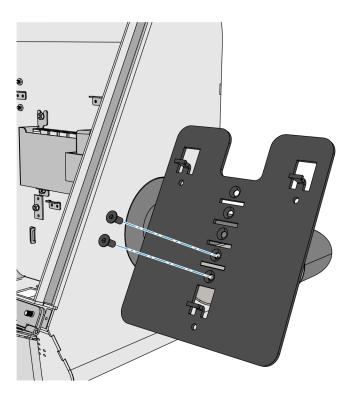
6. Ensure that the left edge of the adapter plate is straight and parallel to the right edge of the cabinet.. Otherwise, adjust the tilt arm until the adapter plate is straight.
