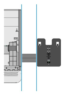
7. Mount the PIN pad on the adapter plate. Insert the PIN pad mounting holes through the hooks (3) on the adapter plate.
