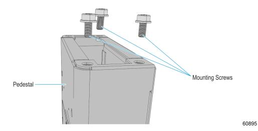
8. Position the kiosk on top of the pedestal with the Mounting Screws (3) extending up through the keyholes in the bottom of the kiosk cabinetand then slide the kiosk cabinet to the right.
