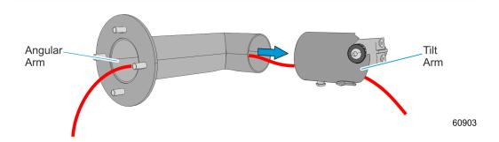
c. Adjust the tilt arm, rotating it clockwise or counter-clockwise, to position the locking screw at the center.
