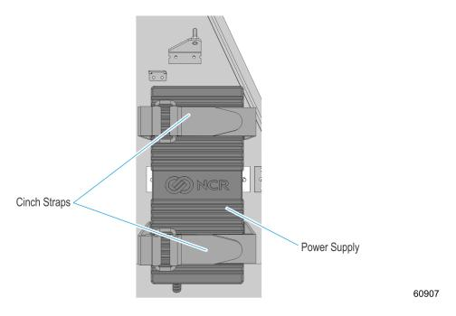
b. Remove the screws (2) that secure the power supply bracket. Remove the bracket.
