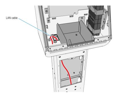
17. Route the LAN Cable towards the motherboard and connect the cable to the LAN port. Secure the LAN cable along with other cables in its path with cable ties as necessary.
