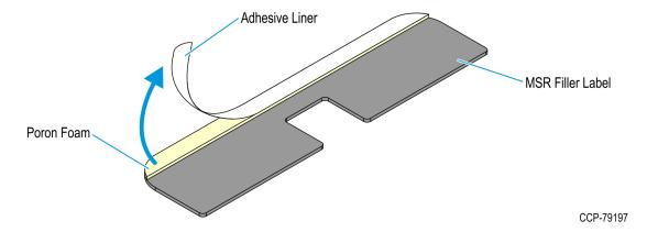
2. With the Poron Foam on the right-hand side, insert the Filler Label into the slot in the MSR device.
