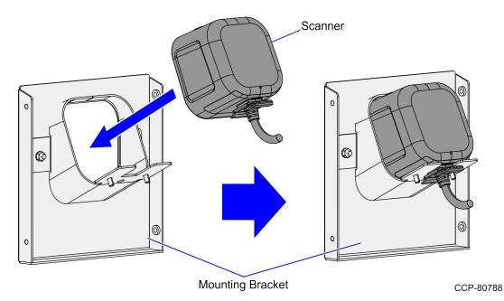
3. Using two (2) wing nuts, secure the Scanner on the Front Housing with the Scanner Mount, as shown in the image below.
