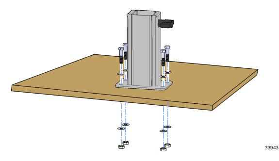
4. Remove the Thumbscrew and the Front Cover from the Checkstand Mount.
