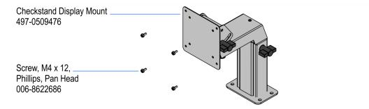
**Note:** The screws in the kit are for XL Displays (5910/5915). For X-Series Displays (5968/5985), use screws included with the display.
