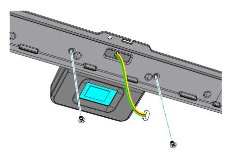
6. Route the Capacitive Biometric Reader Cable through the Cable Guide on the Display Collar.
