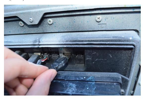
5. Route and plug in the Printer Power cable to the DC power board inside the dispenser.
