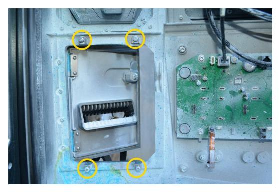
b. Slide the printer assembly onto the support screws.
