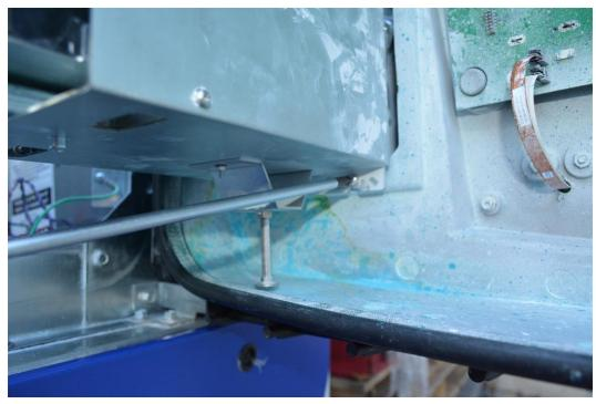
d. Make final support rod adjustments. The support rod should be adjusted so it sits on the bottom edge of the dispenser door. Loosen the rod from the printer chassis until it touches the bottom of the door and meets slight resistance. To keep the rod in place, tighten the nut against the bottom of the printer chassis.
