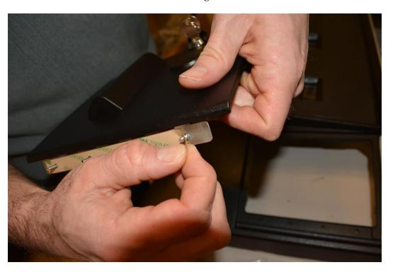
2. Attach the hinge to the right side of the door and secure with the 4 provided nuts (006-8611952) on the back side of the dispenser door.
