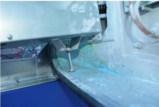
c. Tighten the 4 support screws.
