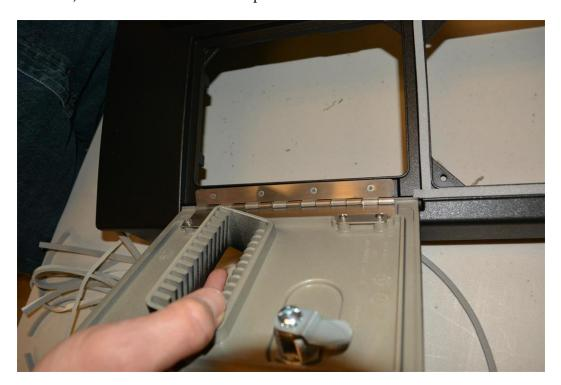
3. Install the gasket (497-0514265) over the side of the hinge making sure the gasket stays within the channel in the dispenser door. Orient the gasket so the thick side of the gasket covers the hinge.
