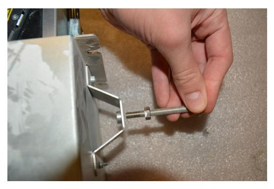
c. Adjust the support rod so the Reuse Printer Assembly can be installed. The support rod should be able to just clear the bottom edge of the dispenser door. Adjust the rod by turning the nut towards the bottom of the support rod and then tightening the rod deeper into the printer chassis.
