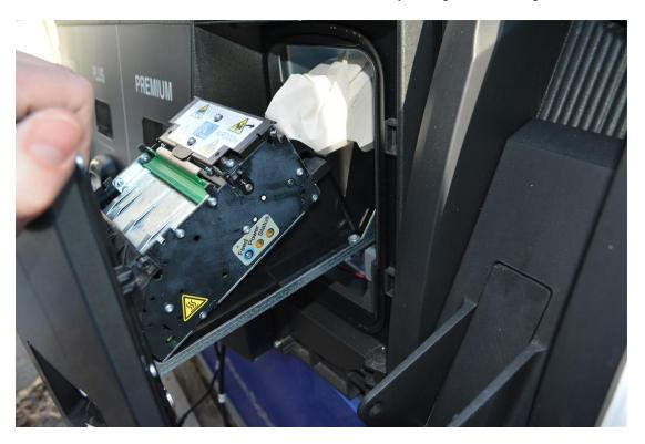
2. Unplug the printer from the interior components and DC power board.
