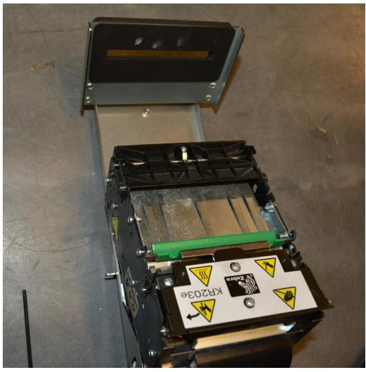
c. Slide the printer forward on the Reuse Chassis until the front of the printer mates up to the gasket shown and engages the Chassis snap.
