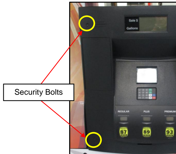
Fig 1 – location of security bolts
