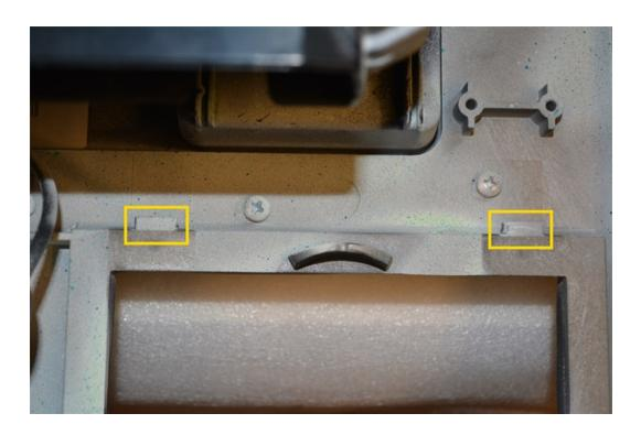
b. Install the provided screws (006-8611475) in the lower section of the printer assembly and attach to the Helix OPTIC 12 panel.
