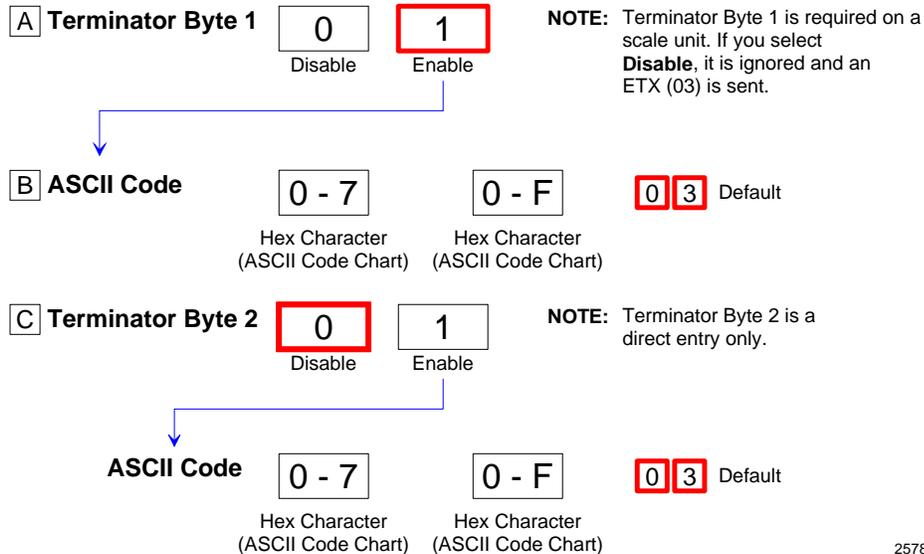
The RS232 Terminator Byte programming mode controls the use of terminator bytes. If an RS232 Terminator Byte is used, it goes at the end of the message sent to the host terminal. If a BCC is included, it follows the Terminator Byte and includes the Terminator Byte in the calculation. Refer to the *Parameter Defaults* section earlier in this chapter for the factory defined default value of each programming parameter.
