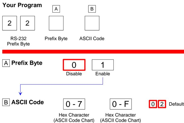
The RS232 Prefix Byte programming mode controls the use of prefix bytes. If an RS232 Prefix Byte is used, it is the leading character in each message sent to the host terminal. Following it is the message data. Refer to the *Parameter Defaults* section earlier in this chapter for the factory defined default value of each programming parameter.
