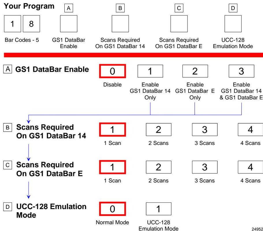
The Bar Codes 5 programming mode contains programming parameters for GS1 DataBar bar codes. Refer to the *Parameter Defaults* section earlier in this chapter for the factory defined default value of each programming parameter.
