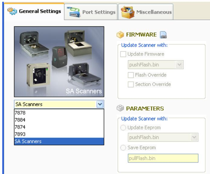
9. Select **Modify INI** after a scanner model has been chosen. Select the **Update Firmware** checkbox and choose the firmware BIN file you want to flash to the scanner. For your preference you may enable Flash Override and Section Override by selecting their checkboxes. Select **Save** to save and apply these settings.
