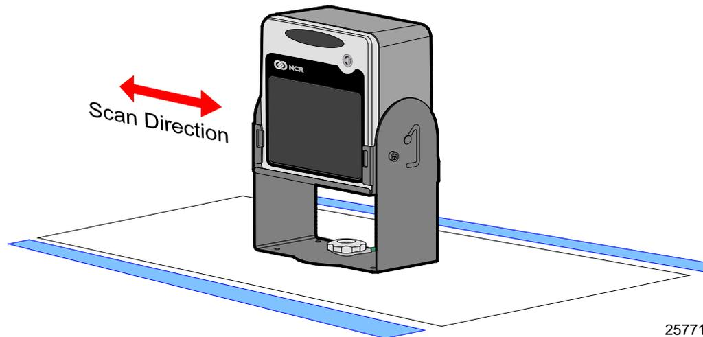
The following image displays the proper scanning direction for horizontal mount configuration.
