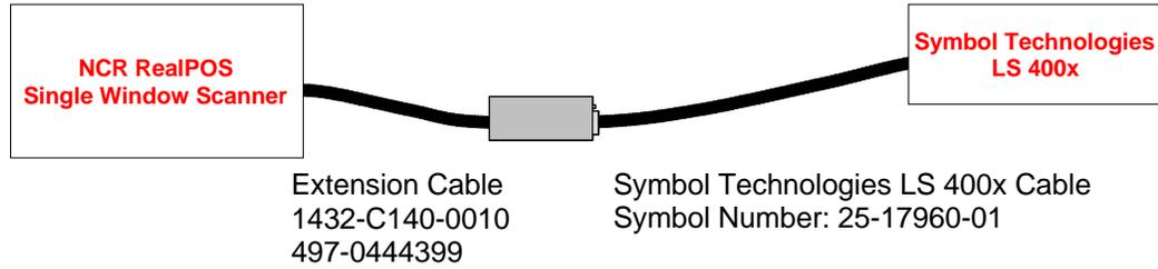
**Note:** The Extension Cable is not required, but can be used if additional cable length is needed.
