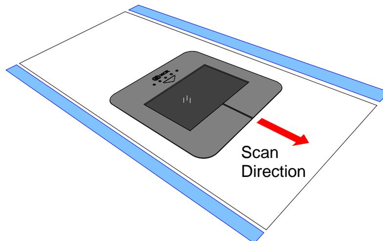
Product labels are read from left-to-right or from right-to-left in the vertical position. When the NCR 7884 is installed using the Vertical Mount, the scan direction is dependent on the mounting position of the scanner.
