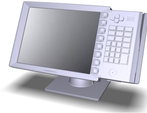
The NCR RealPOS 5954 USB DynaKey is a Point-of-Sale (POS) keypad with a built-in 15-inch flat panel Liquid Crystal Display (LCD). Unique to the DynaKey is a set of ATM-style keys (DynaKeys), which are located beside the display. The functions of these keys change depending on the software application appearing on the LCD.
