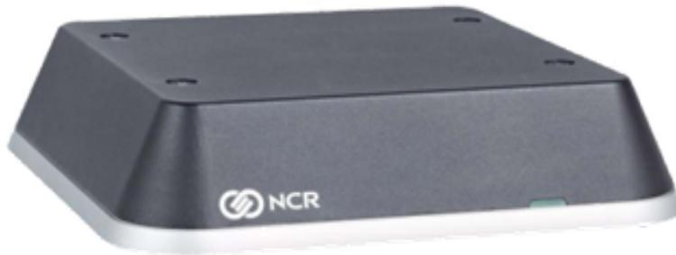
The *NCR Mobile Gateway Controller (MGC)* is a smart controller with pre-loaded software that provides mobile devices access to traditional retail peripherals, including scanners, cash drawers, payment MGCs and receipt printers. It can also be fitted with a stand to hold a mobile device. The MGC can be conveniently and unobtrusively placed throughout a store to handle transactions and service shopper's needs beyond just a tablet alone.
