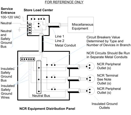
NOTE: NCR Circuits Must Be Dedicated to NCR Equipment or Other Logically Connected Electronic Equipment (Modems, DAA, Bridges, Etc.)
